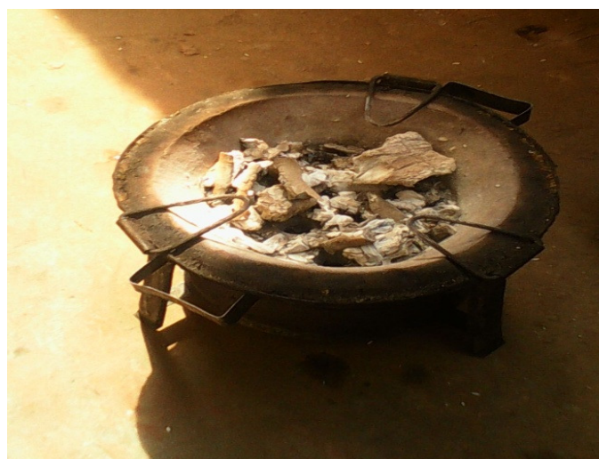
Figure-6 Improved Cookstove with Inner Lining
