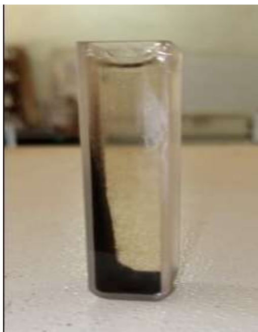
Figure 4. 17: Image of magnetic iron (III) oxide placed near a magnet
