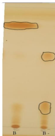
Figure 6. TLC plate after trans-esterification (B: Trans esterified fat & B-: Negative control) (Source: Authors' own elaboration)
