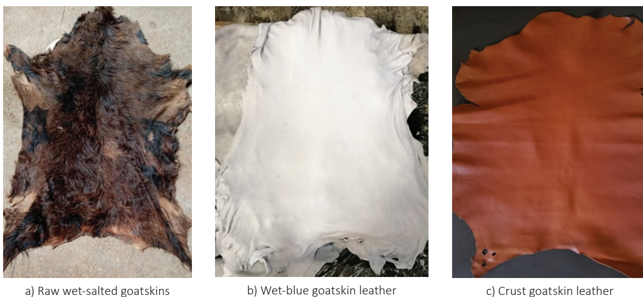
Figure 5. Enzymatically processed goatskin from the raw stage (a), through wet-blue (b) to crust stage (c)
