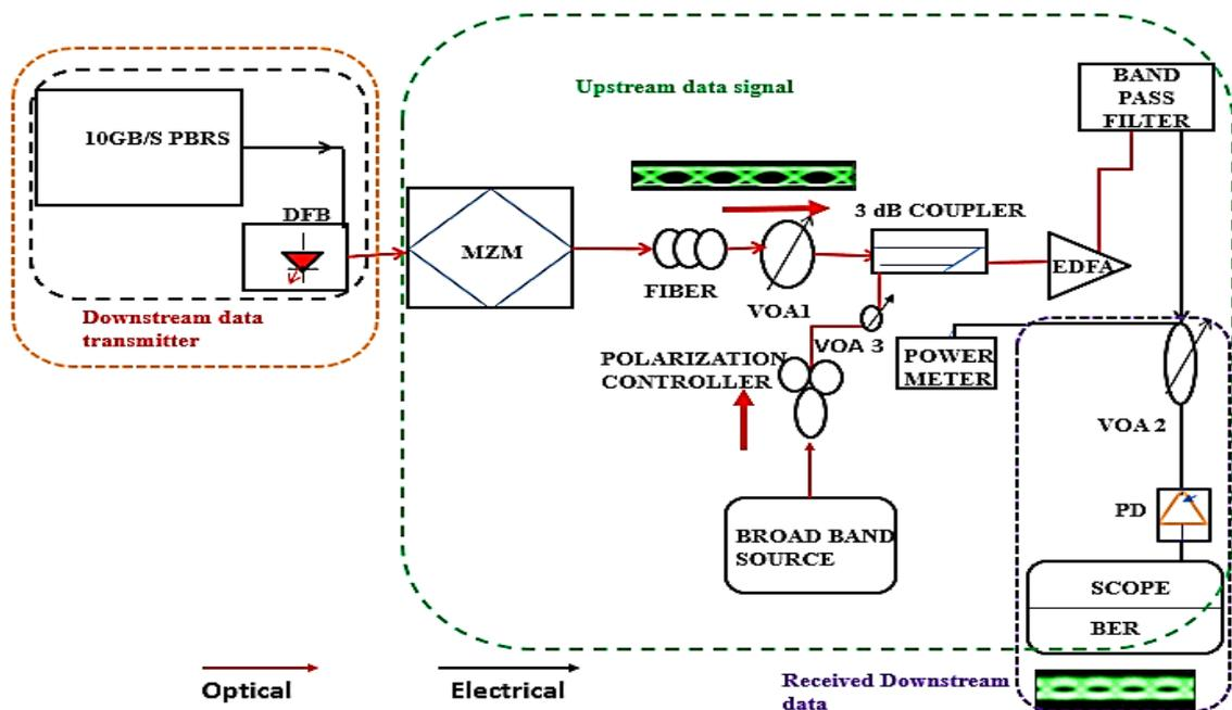
**Figure 3.3:** Experimental schematic illustration of all optical wavelength reuse
