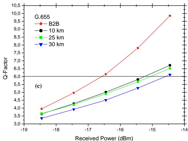
**Figure 4.4 (c):** Simulation variation of Q-factor with received power B2B, 10 km , 25 km and 30 km G.655 1550 nm VCSEL
