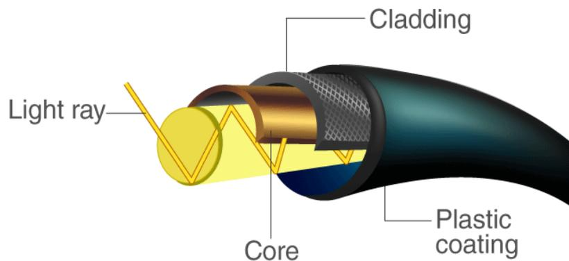
**Figure 2.2:** Components of the optical fiber cable (Wang, 2021)
