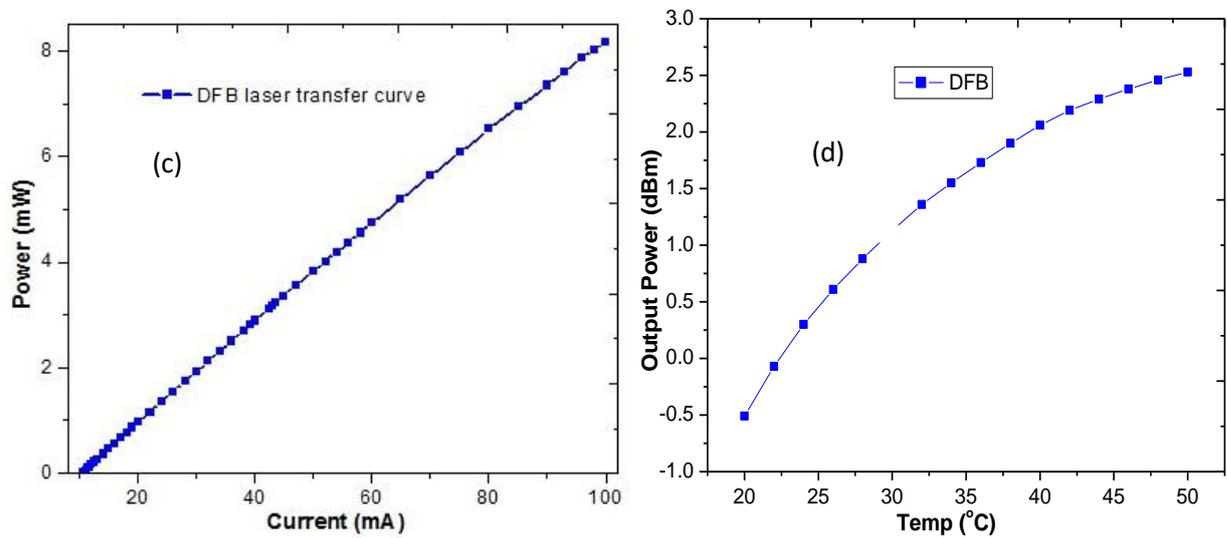
**Figure 4.1 (c):** Input current-output optical power characteristics of DFB measured experimentally at 1550 nm (d) Temperature-power characteristics of DFB at various temperatures.
