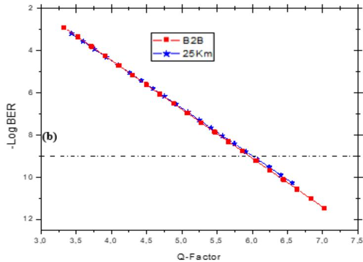
**Figure 4.4 (b):** Plot of -Log (BER) as a function of Q-factor
