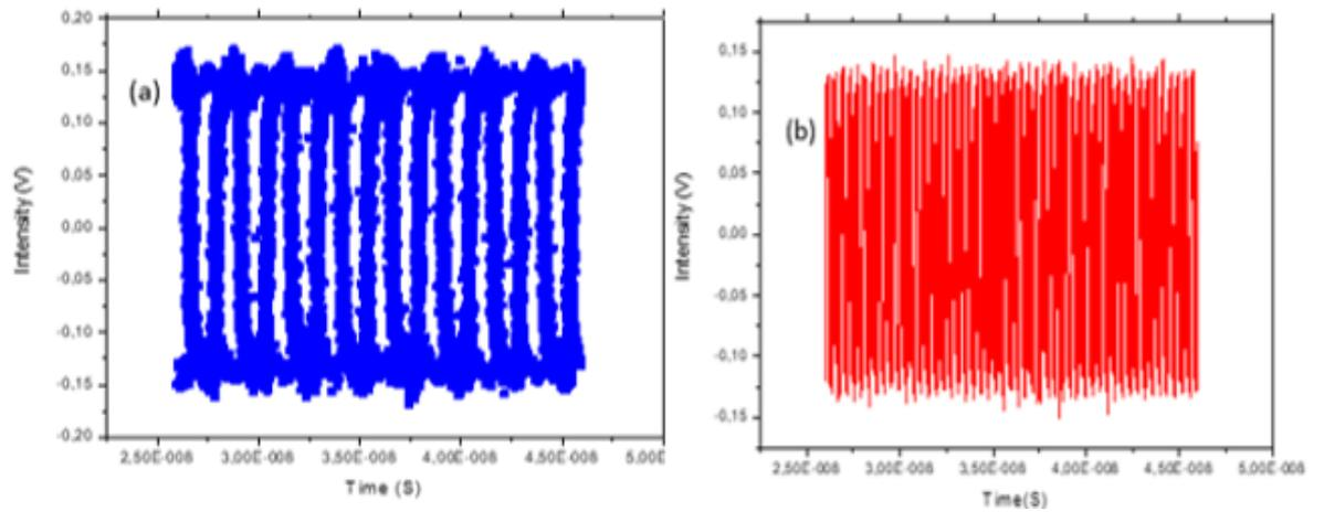
**Figure 4.6:** Electrical clock signal at a frequency of (a) 0.4 GHz (b) 2.5 GHz frequency
