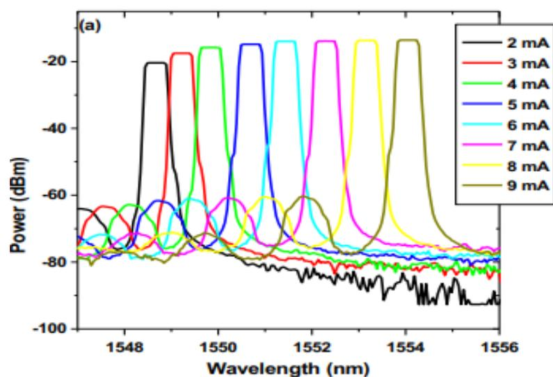
**Figure 4.1 (a):** Wavelength tunability of VCSEL with bias current
