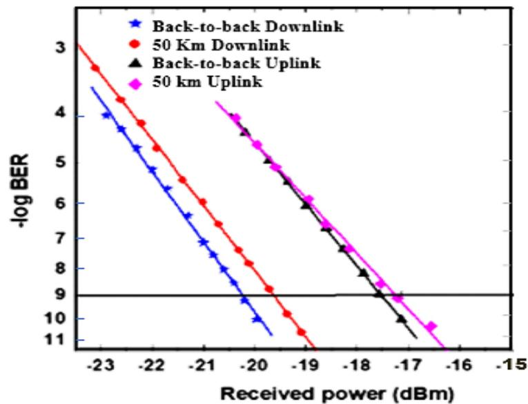
**Figure 4.9:** Experimentally obtained BER curves with EDFA gain saturation for B2B, 50 km downlink transmission and B2B, 50 km uplink (after data erasure) transmission. In uplink transmission, the incident power for B2B and 50 km transmission measurements at  $10^{-9}$  threshold were recorded as -17.48 dBm and -17.02 dBm
