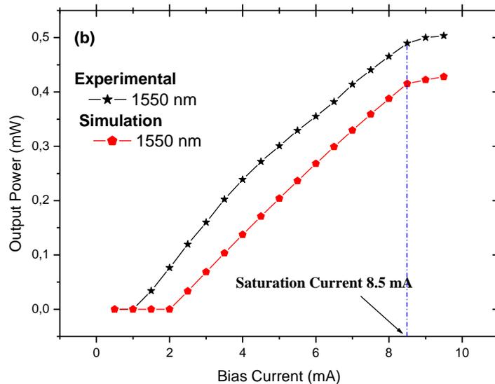
**Figure 4.1 (b):** Measured input current-output optical power characteristics of VCSEL at 1550 nm based on simulation and experiment
