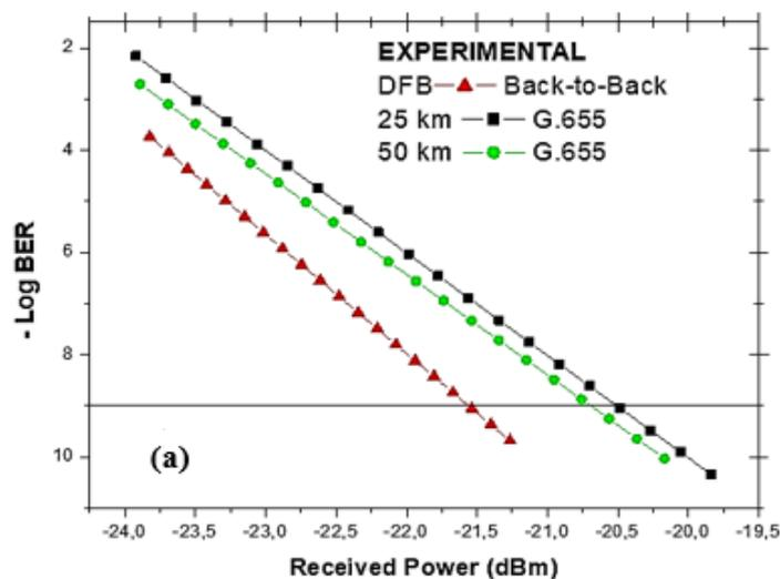
**Figure 4.3 (a):** Experimental  $-\text{Log BER}$  curves for 25 km and 50 km WDM DFB transmission on a G.655 fiber
