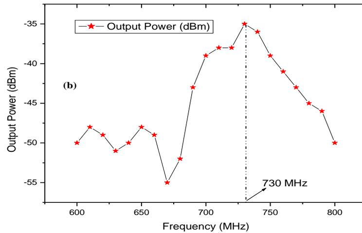
**Figure 4.11 (b):** A graph of output power Vs frequency for the LoRa TTGO ESP 32 Dev module
