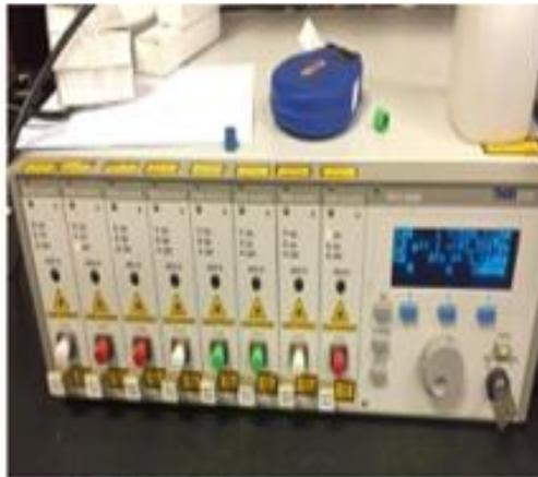
A PRO 8000 WDM laser transmitter source from THORLABS
