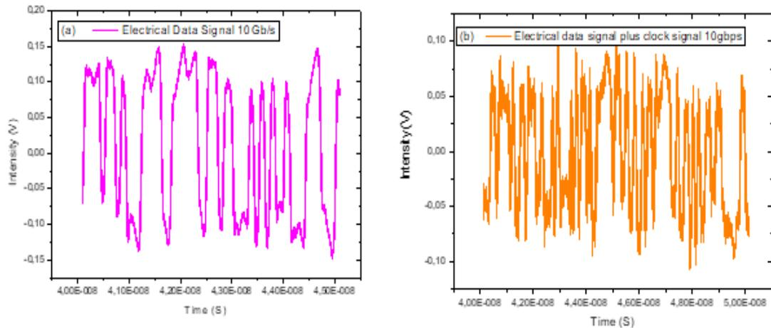
**Figure 4.7:** (a) A graph of 10 Gbps data signal sent over 25 km fiber using a VCSEL
