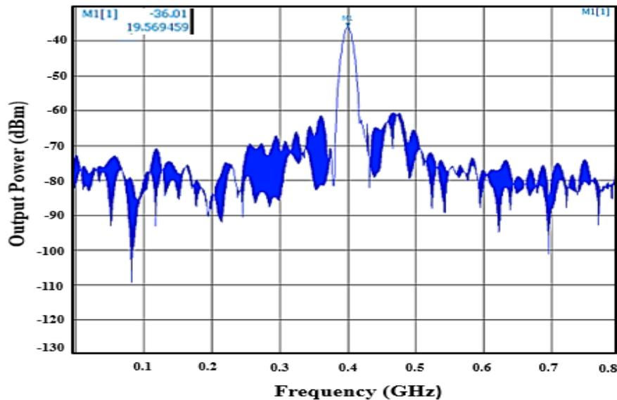
**Figure 4.5:** Experimentally measured electrical clock signal spectrum at 0.4 GHz
