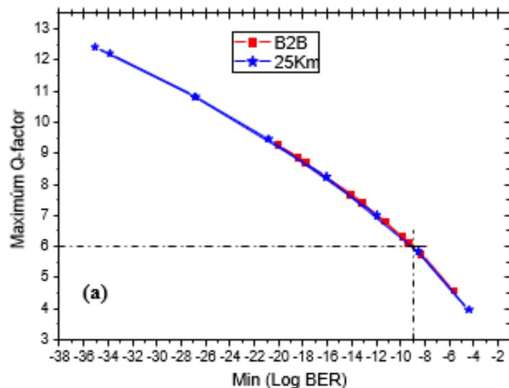
**Figure 4.4 (a):** Plot of Q-factor against min log BER B2B and 25 km G.655
