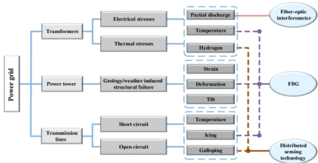
**Figure 2.3:** The smart grid structure and fiber optic sensing technology (Chai et al., 2019)
