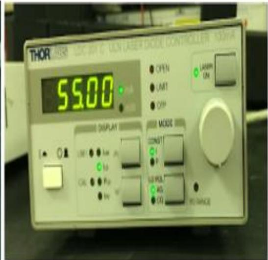
Laser Diode Controller (LDC)
