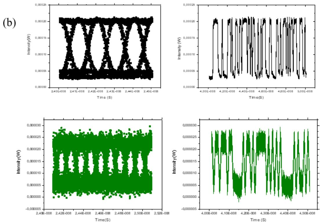
**Figure 4.3 (b):** Eye diagrams and resultant waveforms for 25 km (black) and 50 km (green) transmission using a DFB
