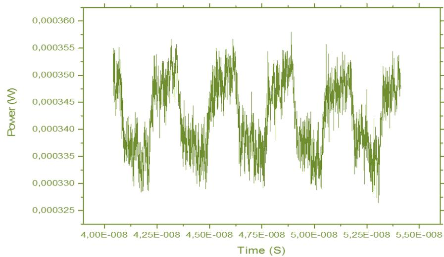
**Figure 4.14:** LoRa-VCSEL B2B output signal before electrical amplification
