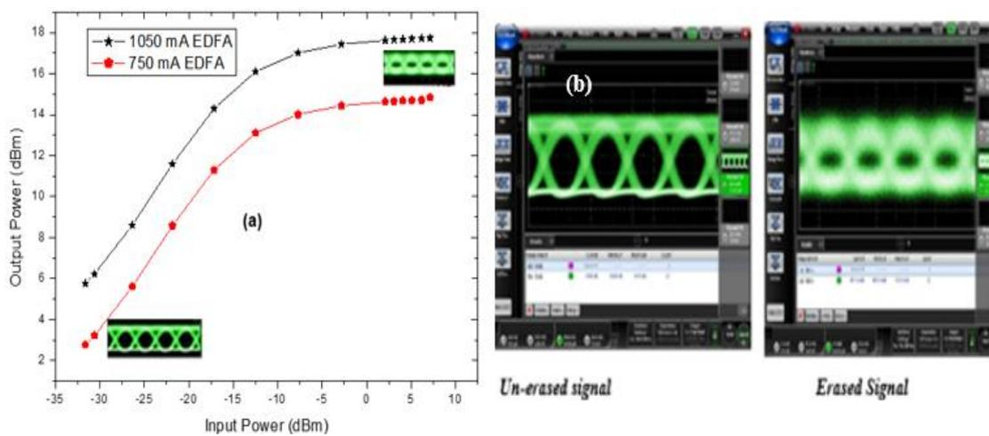
**Figure 4.8:** (a) EDFA characterization at 1050-mA and 750-mA currents (b) analysis of eye diagrams for unerased signal at ER of 9.678 dB and the erased signal with an ER 0.701 dB
