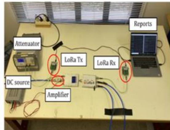
LoRa module experimental setup for signal analysis
