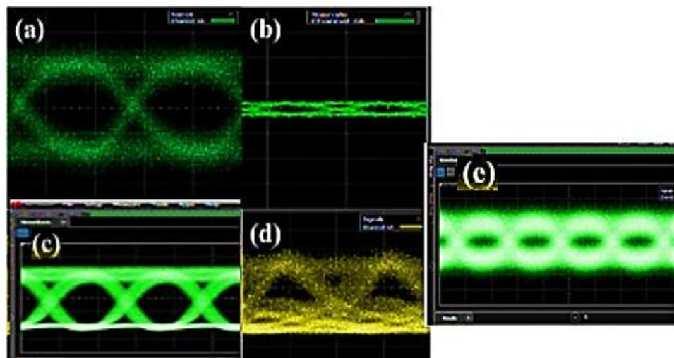
**Figure 4.10:** Eye diagrams measured at (a) B2B ER 7.016 dB, (b) 50 km downstream link transmission ER 5.391 dB, (c) B2B (upstream) link ER 9.678 dB, (d) 50 km (upstream) ER 6.756 and (e) erased channel ER 0.701 dB
