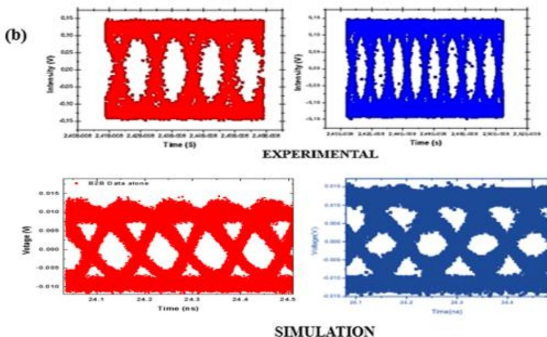
**Figure 4.2 (b):** Experimental and simulated eye diagrams for B2B (Red) and 25 km (blue) transmission using a VCSEL
