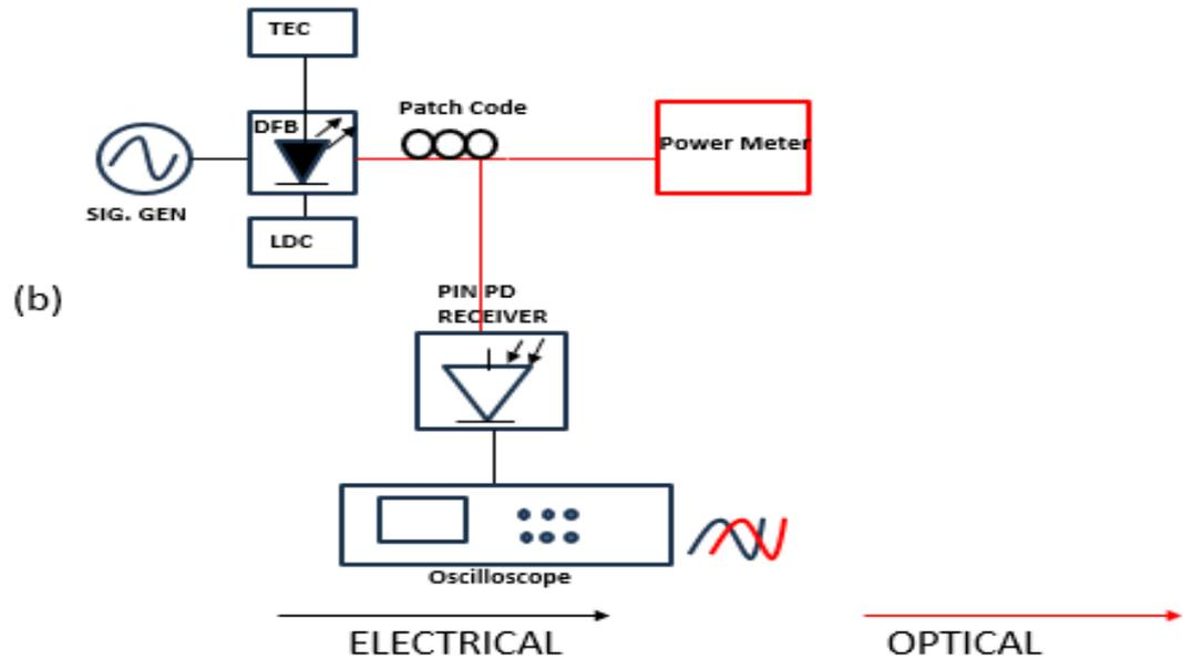
**Figure 3.1 (b):** The experimental characterization of unmodulated DFB laser
