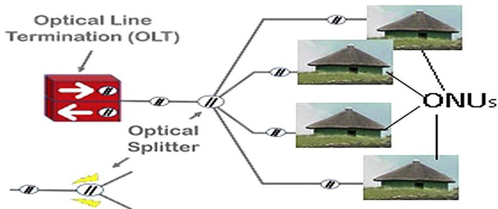
**Figure 2.4:** A schematic diagram of a typical PON representation (Kipnoo et al., 2017)
