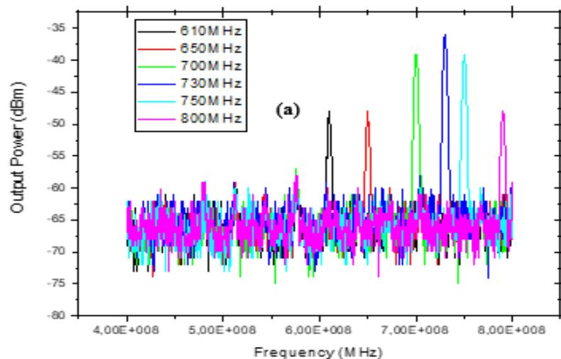
**Figure 4.11 (a):** Experimental frequency characterization of the LoRa TTGO ESP 32 Dev Module
