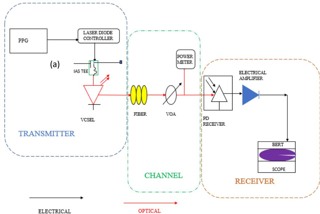
**Figure 3.1 (a):** The experimental characterization set up of a 10 Gbps directly modulated VCSEL
