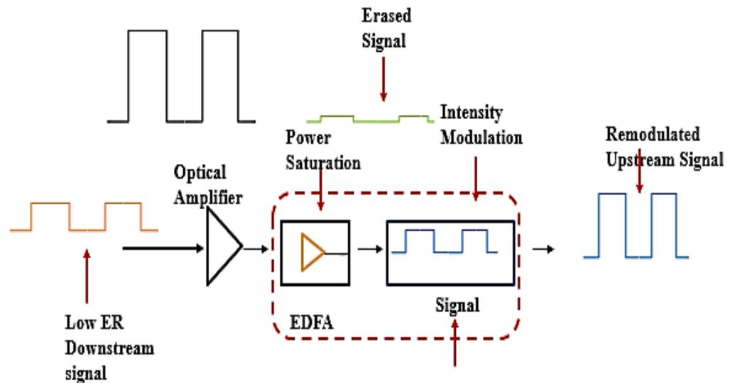
**Figure 3.2:** Wavelength channel data erasure principle
