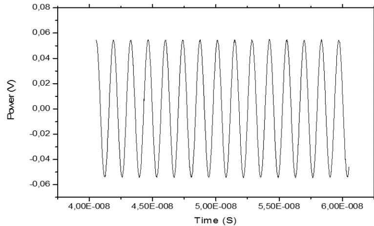
**Figure 4.12:** Optical input signal to LoRa at 730 MHz (signal generator)
