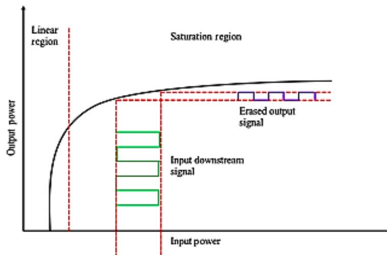
**Figure 2.6:** EDFA characterization used to achieve saturation for data erasing showing the output power as a function of input optical power (Takesue & Sugie, 2003)
