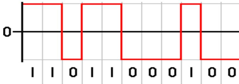
**Figure 2.5:** Data signal format for NRZ modulation (Muthana et al., 2011)
