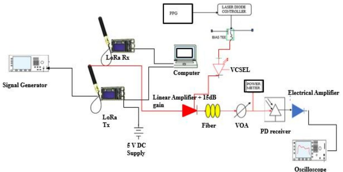
**Figure 3.4:** LoRa module connected for signal analysis on the scope
