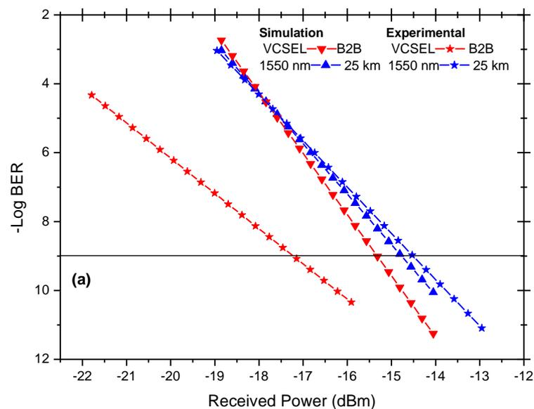
**Figure 4.2 (a):** Simulation and experimental plots of  $-\text{Log BER}$  curves for B2B and 25 km transmission using 10 Gbps 1550 nm VCSEL
