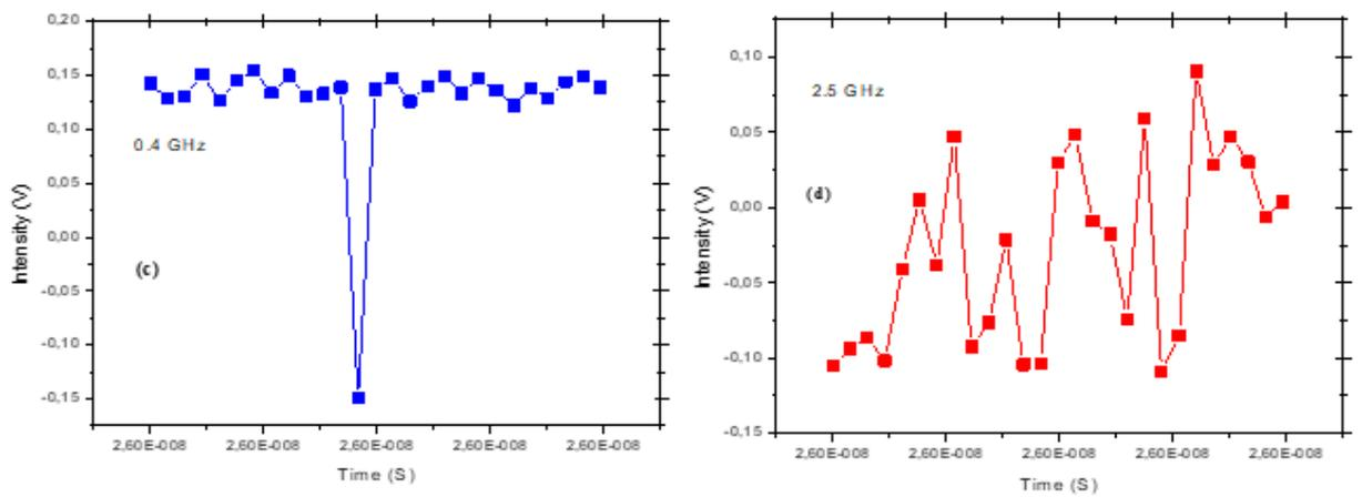
**Figure 4.6:** Sampled 27 transmitted bits in (c) 0.4 GHz and (d) 2.5 GHz
