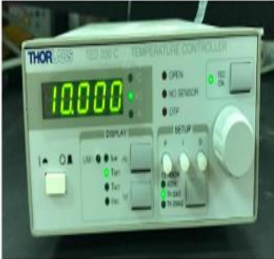
Temperature Stabilizer Thermoelectric cooler
