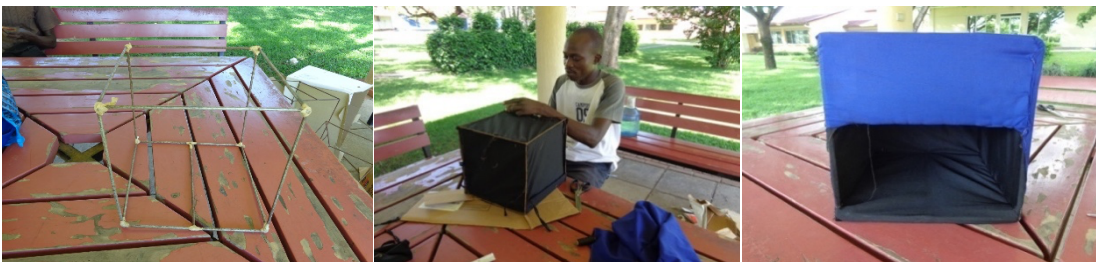
Figure 1 Assembling a simple mosquito resting boxes (modified after Harbison et al., 2006) for indoor resting mosquito sampling
